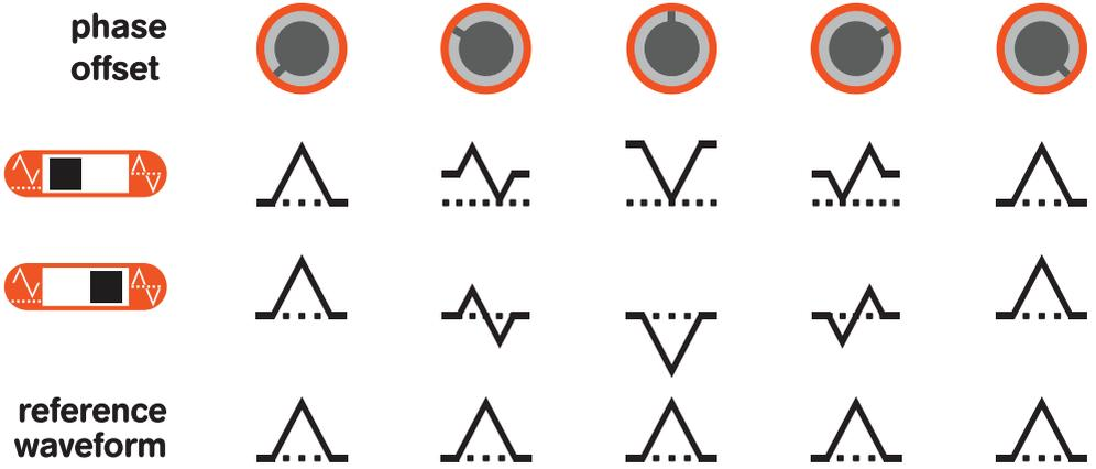
Figure 1b shows how phase offset affects the outputs when attack and decay rates are not equal.
